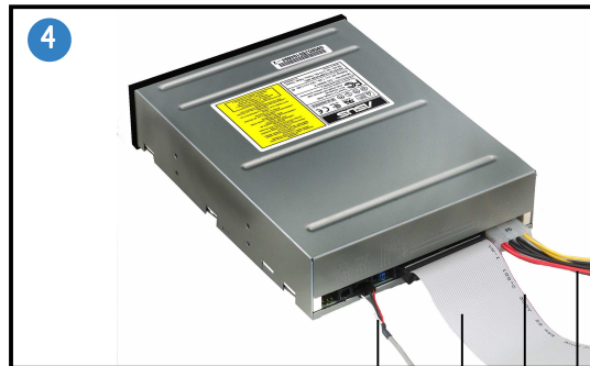
Audio cable IDE ribbon cable Red stripe to pin 1 Power cable
